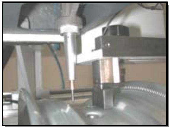
**ML 135/M** – Wheel control bench and manual truing for motorcycle wheels. The machine is supplied complete with N. 1 set of tailstocks for one kind of hub
