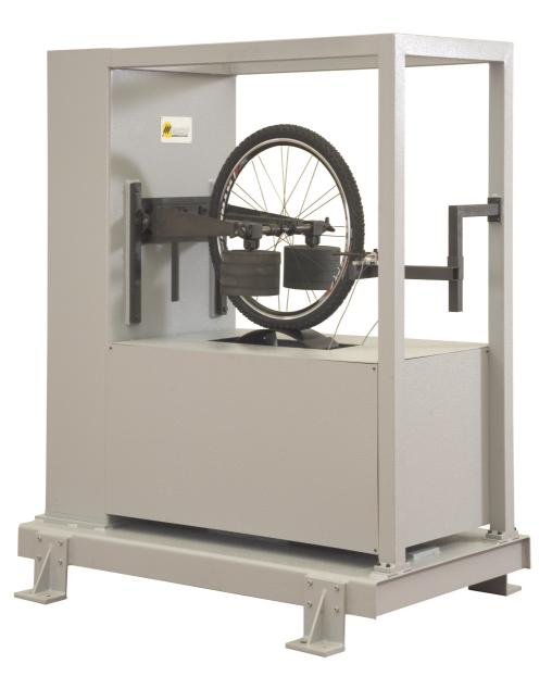
MACHINE FOR THE WHOLE TESTING ON BICYCLE WHEEL ON THE BASIS OF THE FOLLOWING EUROPEAN STANDARDS EN 14764 - CITY AND TREKKING BICYCLES
