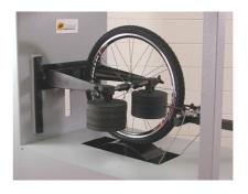
The machine is composed by the following groups: FE Electrowelded base Personal Computer with possibility to memorize all the data Adjustable speed Automatic control with electronic sensor stop the test Set up Time : 5 min. Range : 12"-28"
