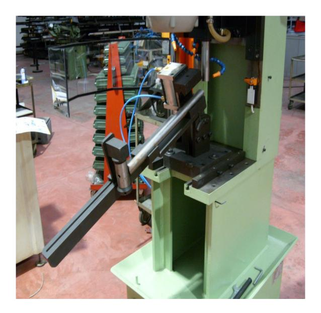
TOOL UNIT FOR MITRING FRAME FRONT DIAMOND TUBES WITH PNEUMATIC LOCK
