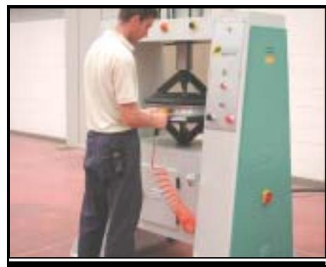
**ML 113/M** - Semi-automatic spoke-tensioning machine. Very strong equipment, compact and sturdy, offering linear design and flexibility of operation.
