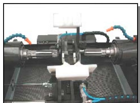
Highly compact and heavy duty machine, made up of two main oleopneumatic groups suitable for reaming (or repassing) the BB shell hole, for tapping (or repassing) the thread and subsequently for facing the shell, so as to ensure that the threads are precisely in axis vis-à-vis the BB shell (an essential operation for facilitating correct and accurate assembly of the crank set).
