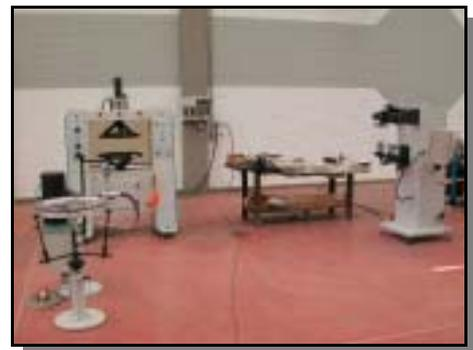
**ML 157M** Wheel assembly station with automatic nipple feed
