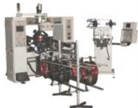
**ML 113/SMN** Electronically controlled spoke tensioning and wheel centring machine for motorcycles and bicycles with four inclinable and adjustable screwing heads
